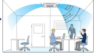
• With Auto airflow direction mode, flaps are controlled to deliver optimal airflow when the room is unoccupied.
